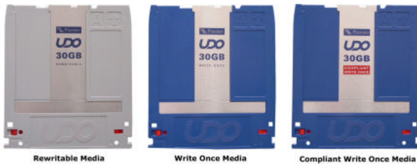
Figure 1 – Photograph of the three UDO media types
