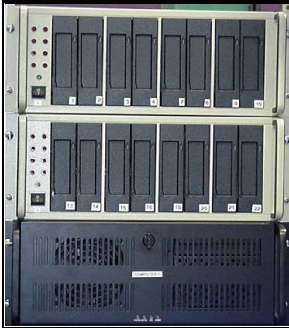
Figure 1: Read/Write Test Fixture
